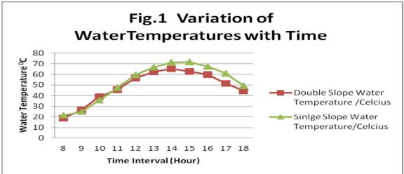
From the figure 1 above, it is categorically clear that, both the two curves have same orientation. This shows that the variation of water temperatures with time has no any physical effect on the performance of solar stills. In other words, the number of slopes in solar stills has no any effect on the variation of water temperature with time.
